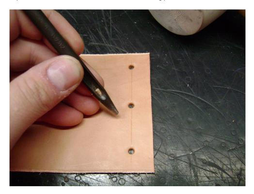
I've again used my binder clips to show the frog part, this time bent around like it will be when attached. I'm going to line it up where I want it on the belt loop and mark through the holes I just punched right onto the belt loop piece, to show where it'll be riveted onto that piece. Make sure you're tilting it the right way – this one is a right-handed draw.
