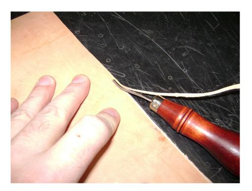
Here's what a beveled edge should look like. I didn't bevel the ends of the frog piece. There's no need to there, we're butting those pieces together in an unseen area. Notice the nice, rounded edge. Try and duplicate this with your utility knife. Use your carpenter's square for a straight edge guide if it helps.
