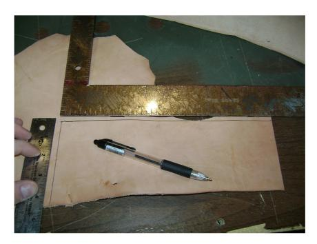
Cut that out, and then square it off. I'm using my leather shears to cut; you should be using your utility knife.
