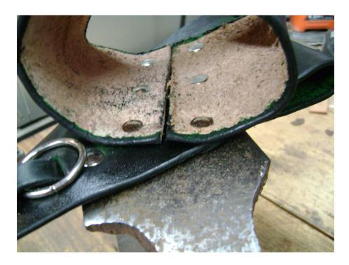
Finally, use two more rivets to attach the two halves of the belt loop together. Just bend the frog leather out of the way to hammer them down if you need to.
