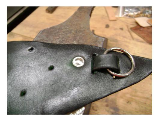
Now you'll attach the frog to the belt loop. Take the belt loop piece, and push six rivet posts up through the holes you punched in the back side.
