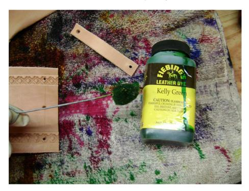
Dip the dauber into the dye, and brush it on. The key here is to really slop it on – don't be stingy with your dye. Give it several coats on the front, a couple on the edges, and give the back a coat too. I don't usually dye the entire backs of things, but some think it looks better if you do, so go ahead if you want to. Make sure if you're not dying the backs that you get a quarter inch or so in from the edge on the backs.
