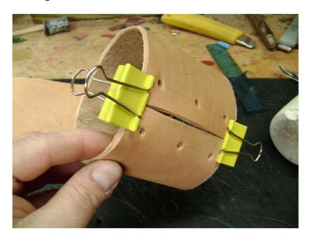
The way this one lay, one of the holes lined up through all three layers of leather. I could move it away, but I happen to have some longer rivets, so I'll use one of them to go through all three layers. You can just move it around until you miss the two holes that hold the belt loop folded over. I stuck a steel scribe tool through all three layers to hold it steady and then marked the other five holes.
