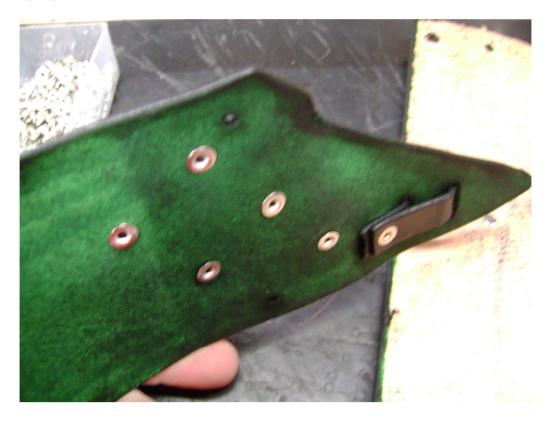
Lay that piece flat on your table, and put the frog piece on top of it, lining up the holes in the frog piece with the rivets sticking out of the belt loop, then press the rivet caps on with your thumb. They should kind of snap into place and hold there. Do one side, then put it on your mini anvil, and use your rivet setter and ball peen hammer to squash the rivet caps down onto the posts.
