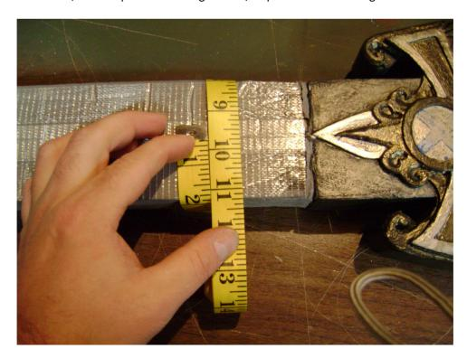
It is about 9 %" around. Using your carpenter's square, mark out a piece 10 %" long by about 4" wide on the leather. This is the part that will hold the sword.
