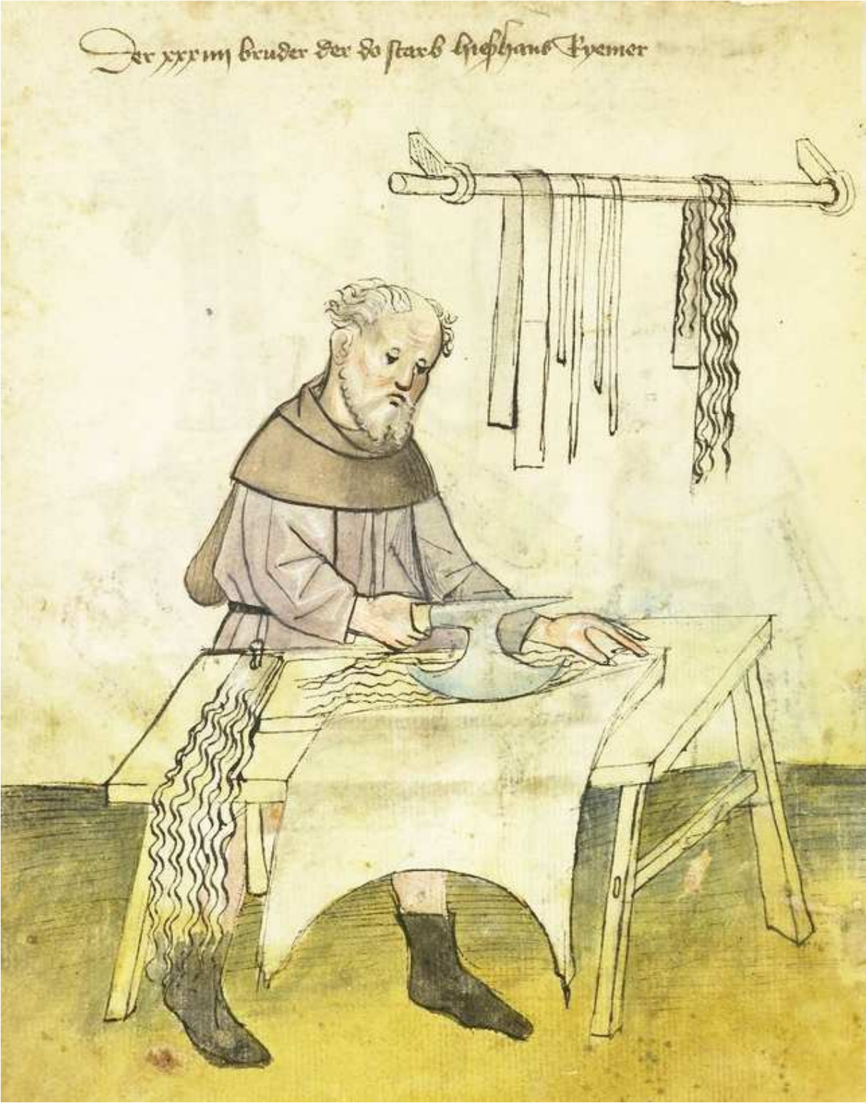
Figure 2: Illustration of a monk using a head knife to cut leather straps, circa 1425. iii
